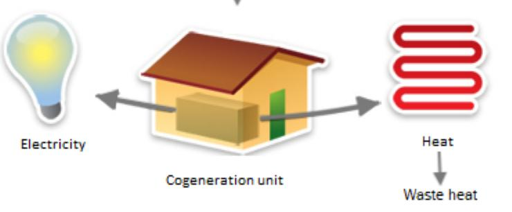
Biogas plants generally use only 20-40 % of the heat that is produced in the cogeneration units and the remaining heat becomes waste heat. Organic compost
